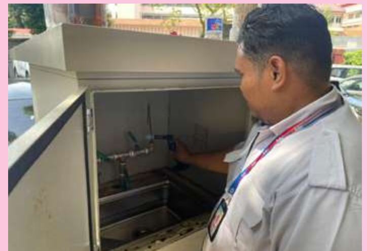
DBKL melaksanakan persampelan air minum di Service Reservoir Outlet Kolam Air Bukit Weld dan Treatment Plant Outlet Loji Bukit Nanas.
